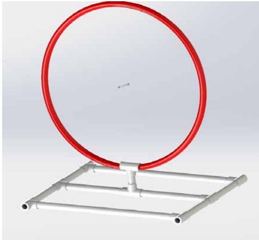
The diameter of the circle is 80 cm and the center of its holder is 10 cm above the ground.
